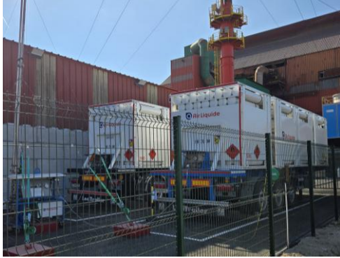
Figure 2. Hydrogen semi-trailers secured by chain-link fencing and mandatory safety clearance distances
